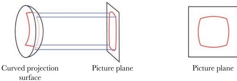
Just as we were able to describe the method of linear perspective projection with a simplified formula, we may do the same for curvilinear perspective. Let  $\text{curv}$  be the projection function for curvilinear perspective, and  $k$  a projective index. Then we may say that the projection function  $\text{curv}$  applied to a scene  $S$  and index  $k$  yields a picture  $P$ :  $\text{curv}(S, k) = P$ .
