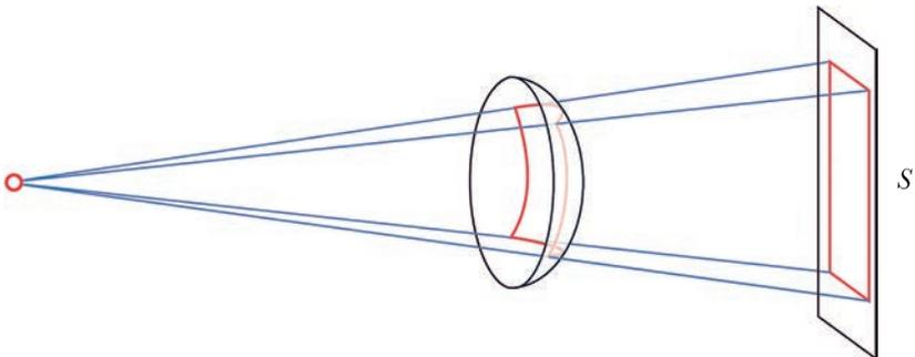
This surface is then transposed onto the picture plane. The result, call it  $R$ , is the product of applying the curvilinear projection function  $\text{curv}$  to  $S$  relative to viewpoint  $j$ . That is,  $\text{curv}(S, j) = R$ .
