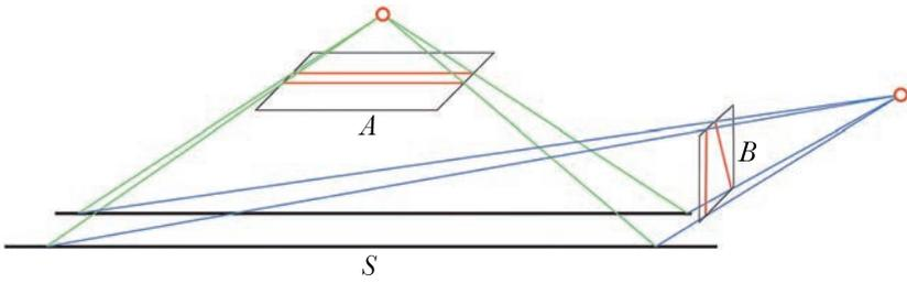
The results of each projection are shown below. Image *A*, produced from the parallel picture plane is a characteristic “bird’s-eye view” of *S*. Note how the lines in *A* are parallel, just as they are in *S*. Meanwhile, image *B*, produced from the perpendicular picture plane reveals the “train tracks effect” of parallel lines converging. *A* preserves the shape, though not the size of *S*. *B* preserves neither.
